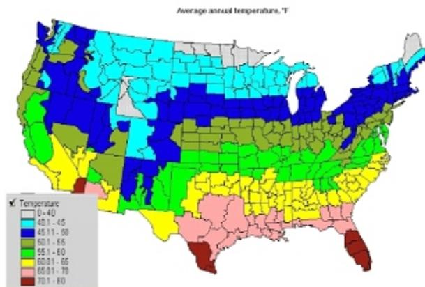
Inlet temperature for most locations exhibits significant daily and seasonal variations. The typical extreme variations have been tabulated by the American Society for Heating, Refrigeration, and Air Conditioning Engineers (ASHRAE). These tables are widely available, and include relative humidity (wet bulb) corresponding to the temperature extremes.
