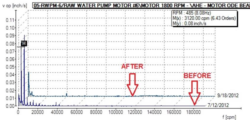
**Motor Vibration Trend & Spectrum Before & After VFD Replacement**
